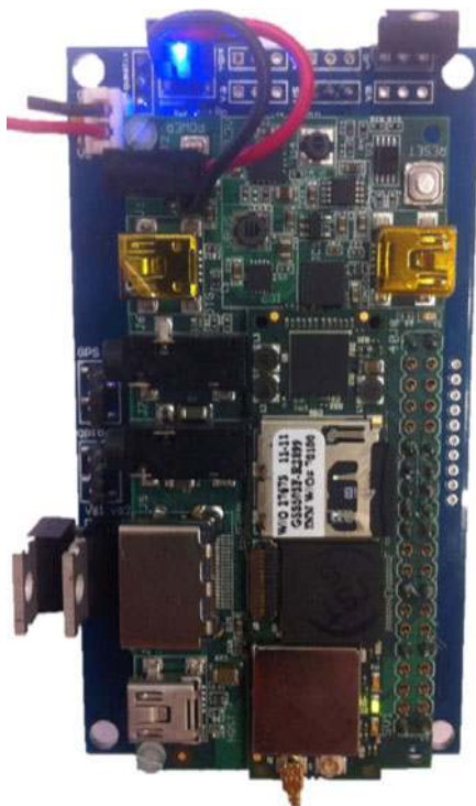
Fig. 8 Gumstix and expansion board
