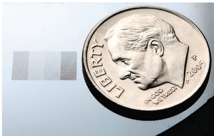
Figure 6. Mirrored pyramidal well array etched on a silicon wafer (with a U.S. dime shown for scale). The pattern on the left contains 2940 wells of three different sizes. Image courtesy of John Russell.
