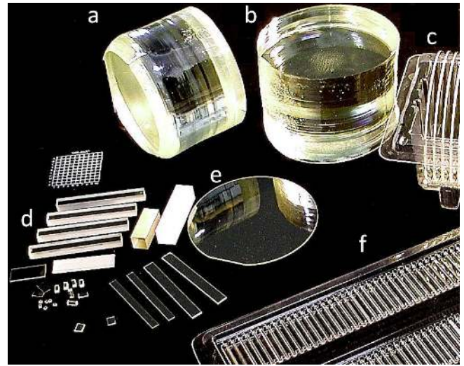
Fig. 1 (a, b) A boule of LN, (c, e) with wafers and (d, f) other shapes cut for typical applications. Image provided by Precision Micro-Optics, MA, USA.
