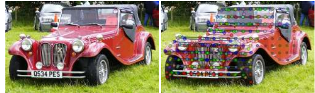
Fig. 8. Illustration of a Micro-HC algorithm for symmetry detection: input photographs and their bilateral symmetry maps. (Ballet photograph courtesy of flickr user dalbera.)
