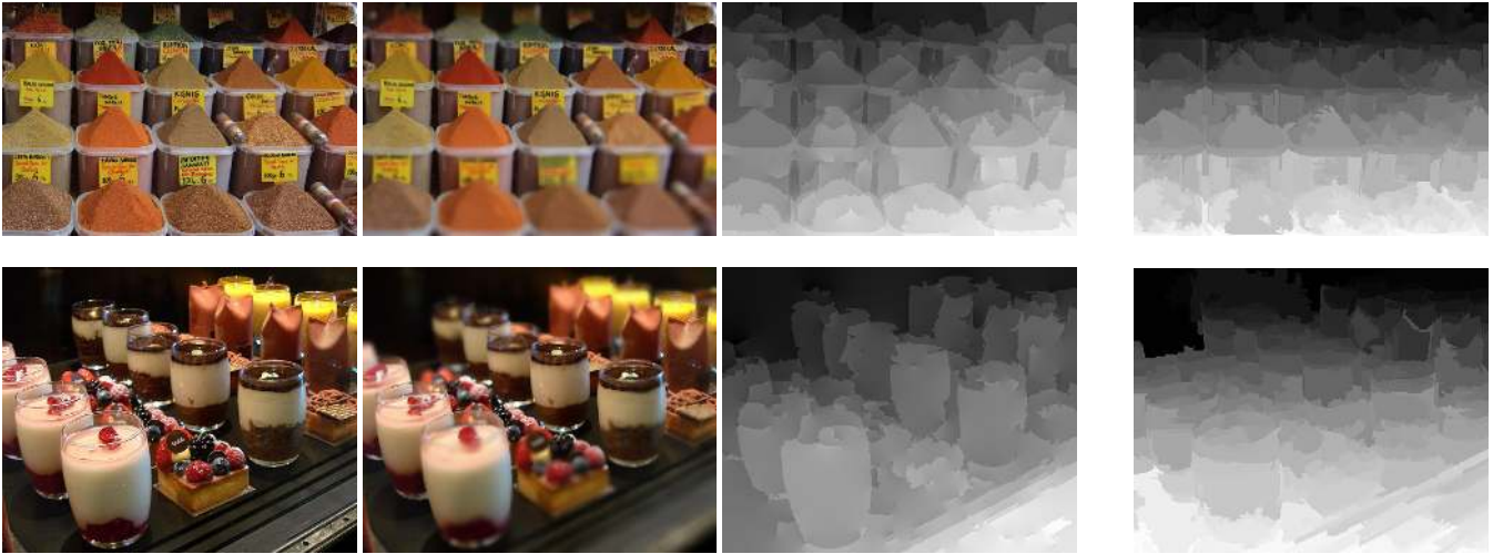
Fig. 4. Results of a Micro-HC algorithm for depth layering: The original photograph (left) & sample application (center-left): using the layers information to apply a depth-based blurring effect. Compare the reconstructed depth layers from HC micro-task results (center-right) to the reconstructed depth map from Make3D [Saxena et al. 2009] (right). Make3D performs well when an image’s depth increases in the up direction and color similarity implies depth similarity (top: spices), but poorly in the absence of these two conditions (bottom: cups). (Original photographs copyright Yotam Gingold.)
