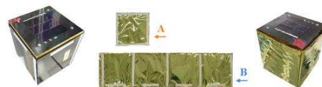
Figure 3. Target Micro Satellites and MLI; (left) Target Micro Satellite Not Covered with MLI, (center) MLI, (right) Target Micro-Satellite Covered with MLI.
