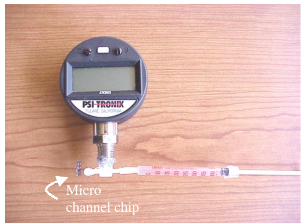
Figure 9. Photograph of the experimental set-up of the quantitative air pressure test.
