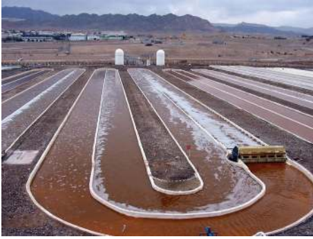
FIGURE 1: High rate algal ponds in Arizona, US (Renewable Fuel and Energy B.V.) [62].
