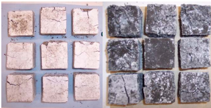
Figure 8. Photographs of 50-mm cubes of MKPC blast-furnace slag (BFS; left) and MKPC fly ash (FA; right), each with a 1:1 ratio of MKPC to diluent, suffering from expansion and cracking 3 days after casting. 208
