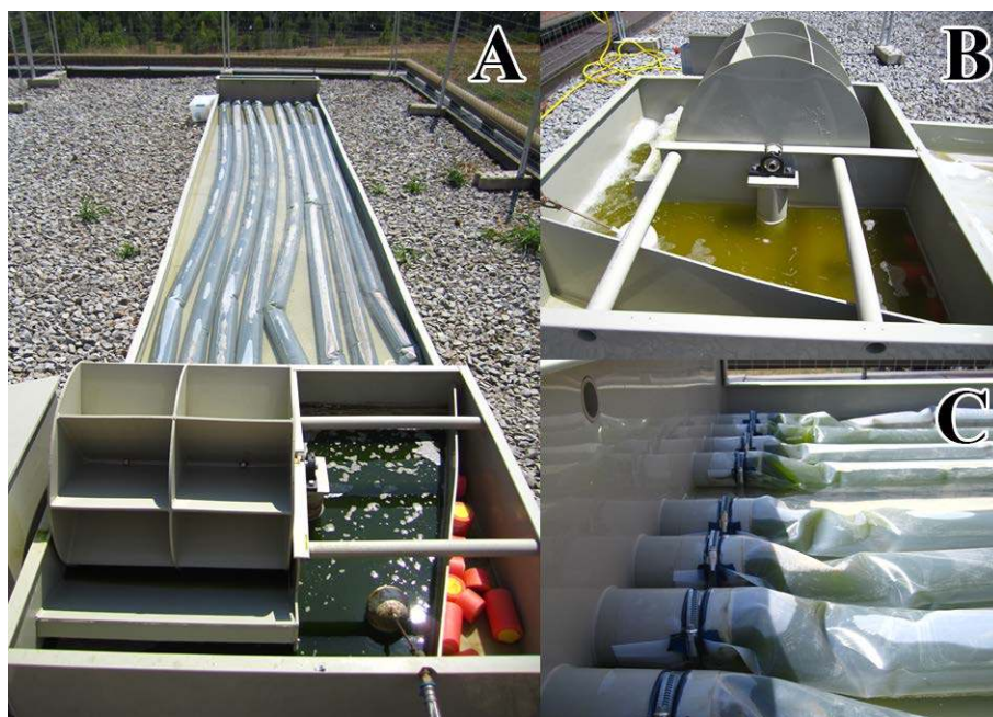
Figure 3.1: Photographs taken during PBR operation. A, General view of the PBR; B, Distribution chamber with the paddle wheel; C, Polyethylene tubes connecting the distribution chambers.
