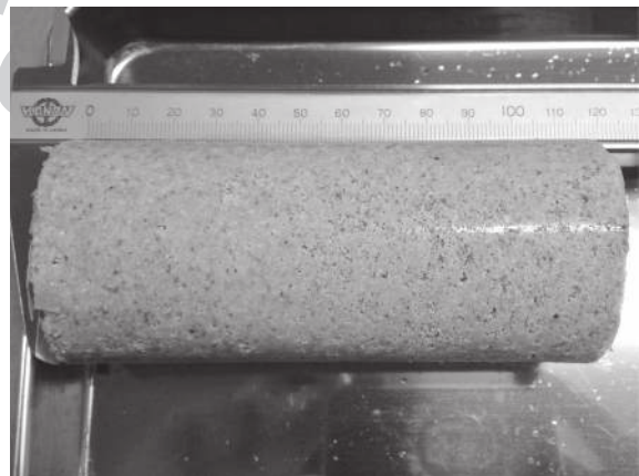
Fig. 16 Column specimen of Case 1 after 28 days of curing (the top of the specimen is positioned on the left and the bottom is positioned on the right).
