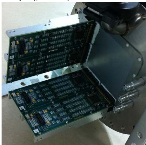
Figure 3. Cross strip detector with ~95 x 95mm aperture. Four 64 channel preamplifiers are shown attached to the detector.
