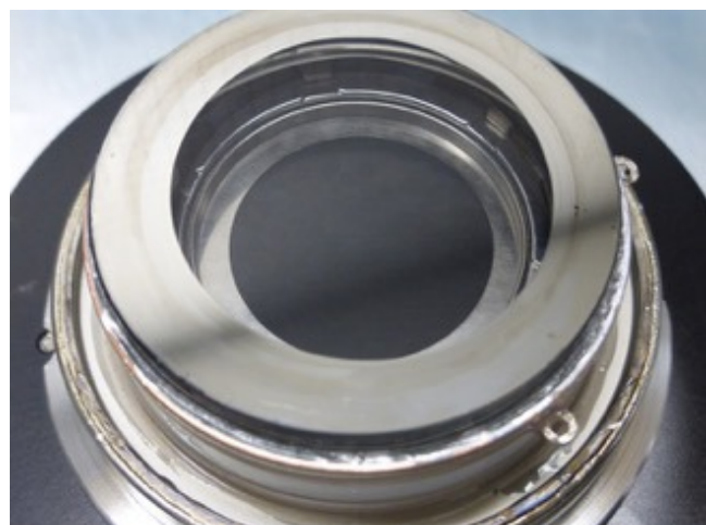
Figure 29. Sealed tube detector with 33 mm ALD MCPs and an opaque GaN photocathode deposited on the top MCP. (20 \mu m pore 60:1 L/d, 8° bias with Al 2 O 3 ALD layer applied).
