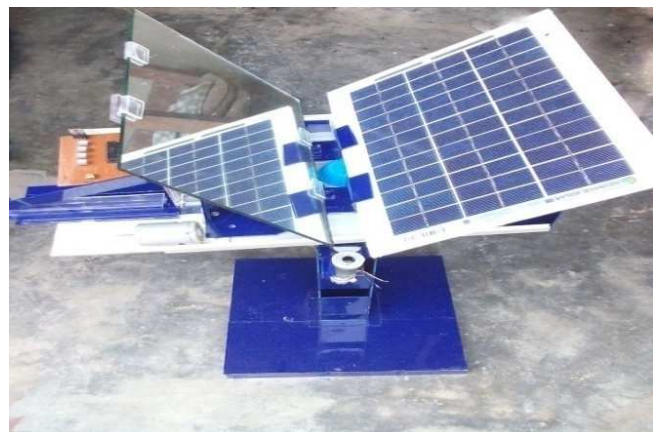
Fig. 10. Mounting the panel on the frame.
