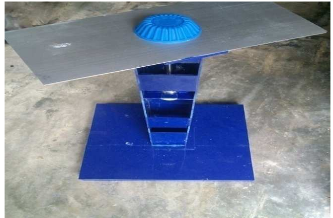
Fig. 9. Foundation of the solar tracker.
