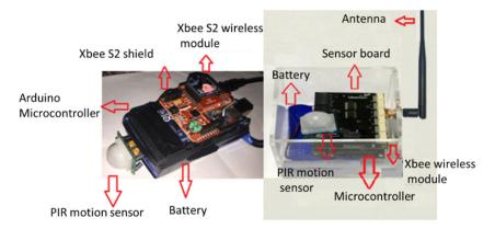
Figure 2. Images of two typical MCU-based wireless sensor nodes [18].
