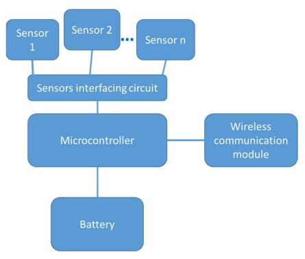
Figure 1. Basic architecture of a sensor node [13].
