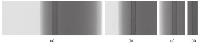
Figure 5: Scans of an aluminium tube placed off-center in a water-filled plastic tube, with scans centered on the aluminium tube, with various degrees of truncation: no truncation (a), and truncated with (b) FOV at 50% width, (c) FOV at 25% width and (d) FOV at 12.5% FOV width. Other intermediate degrees of truncation were also included (not shown).
