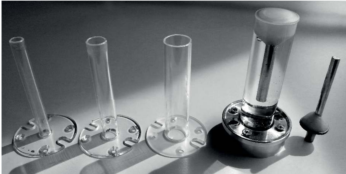
Figure 3: Vertically mounted plastic tubes with inner diameters of 6, 10, 15 and 20mm were water filled and various aluminium rods and tubes were held axially in the tubes as shown. Tubes or rods scanned in air were held on a brass stage by dental wax as shown.
