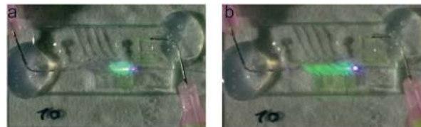
Fig. 5 Characterization of the light focusing principle with different micro-chambers being filled with a solution of fluorescein. Shown in (a) is the reflection of the light towards optical output 2, due to the filling of micro-chambers 1 and 2. Shown in (b) is light being sent through the device, due to the filling of all micro-chambers. Most notable is that the light stops abruptly in (a) due to the TIR at the air interface, whereas full illumination of all micro-chambers is achieved when they are filled with water (b).
