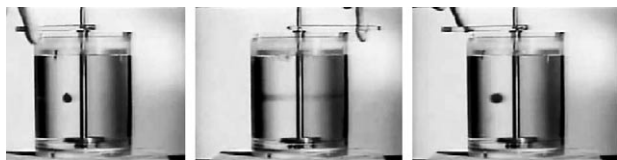
Figure 2. The experiment by G. I. Taylor demonstrates the reversibility of the Stokes equation. A colored droplet is introduced into a highly viscous liquid between two concentric and transparent cylinders (Couette apparatus). When rotating the inner cylinder, the droplet is sheared and therefore smeared. After reversion of the direction of rotation the droplet reassembles again.
