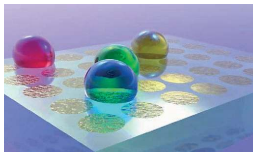
Figure 11. Droplets on a chemically prestructured chip surface. If the droplets are small enough and the surface consists of areas of preferred wettability (hydrophilic anchors), surrounded by hydrophobic regions, the droplets are stabilized at a predetermined volume. They act as individual virtual test tubes for micro-scale laboratories.
