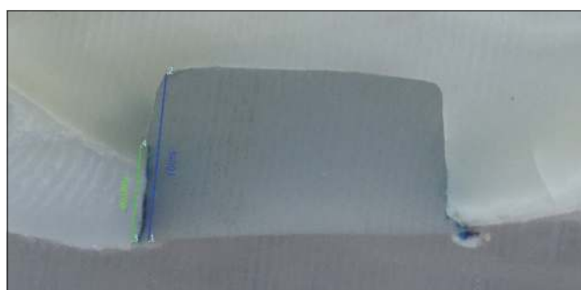
Figure 1: ×40 picture of a sectioned sample with the calculation of the percentage of dye penetration relative to the total length of the restoration interface (100%)
