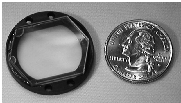
Fig. 10. DMLA color EPE, yielding a uniformity of better than 20% and an efficiency of better than 90% for all colors.
