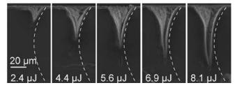
**Figure 3:** Machining of curved trenches in silicon using accelerating beams. In (a) we show the variation in trench properties for different number of passes at fixed energy of 11  $\mu$ J. In (b) we use a fixed number of 5 passes and study the variation in the trench properties with incident energy.
