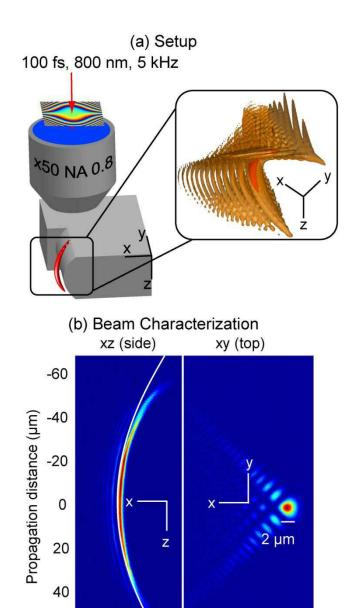
**Figure 1:** (a) Schematic of our experimental setup showing focusing of shaped accelerating beam into our sample. (b) Experimental measurements of accelerating beam profile along direction of propagation i.e. the xz plane in a side view, and viewed from the top in the xy plane at the point of peak intensity at z=0. The white line shows the target circular beam trajectory with radius  $R=120~\mu m$ .
