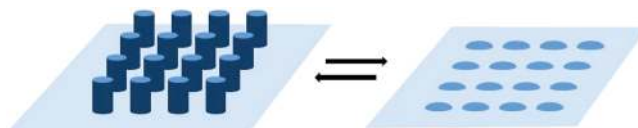
Figure 1. Responsive surface with a stimuli-driven roughness change.
