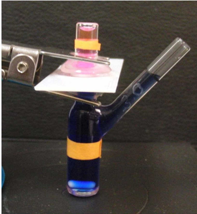
Figure 2. Franz™ Cell diffusion cell (PermeGear, Inc) shown with a pink donor chamber, blue receptor chamber and acrylic holder in place of the membrane. The diffusion cell is held together with a spring bound clamp.
