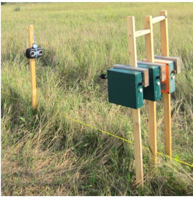
Fig. 2. Experimental setup showing one of 12 triads of autonomous recording units used to evaluate the effect of microphone sensitivity loss on detection of calls. We simulated wind noise by broadcasting 42 dBA and 50 dBA (measured 1 m away) of white noise from a pair of speakers placed in front of each triad.
