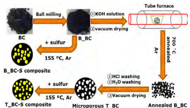
Scheme 1 The preparation process of T BC -S and B BC -S composites
