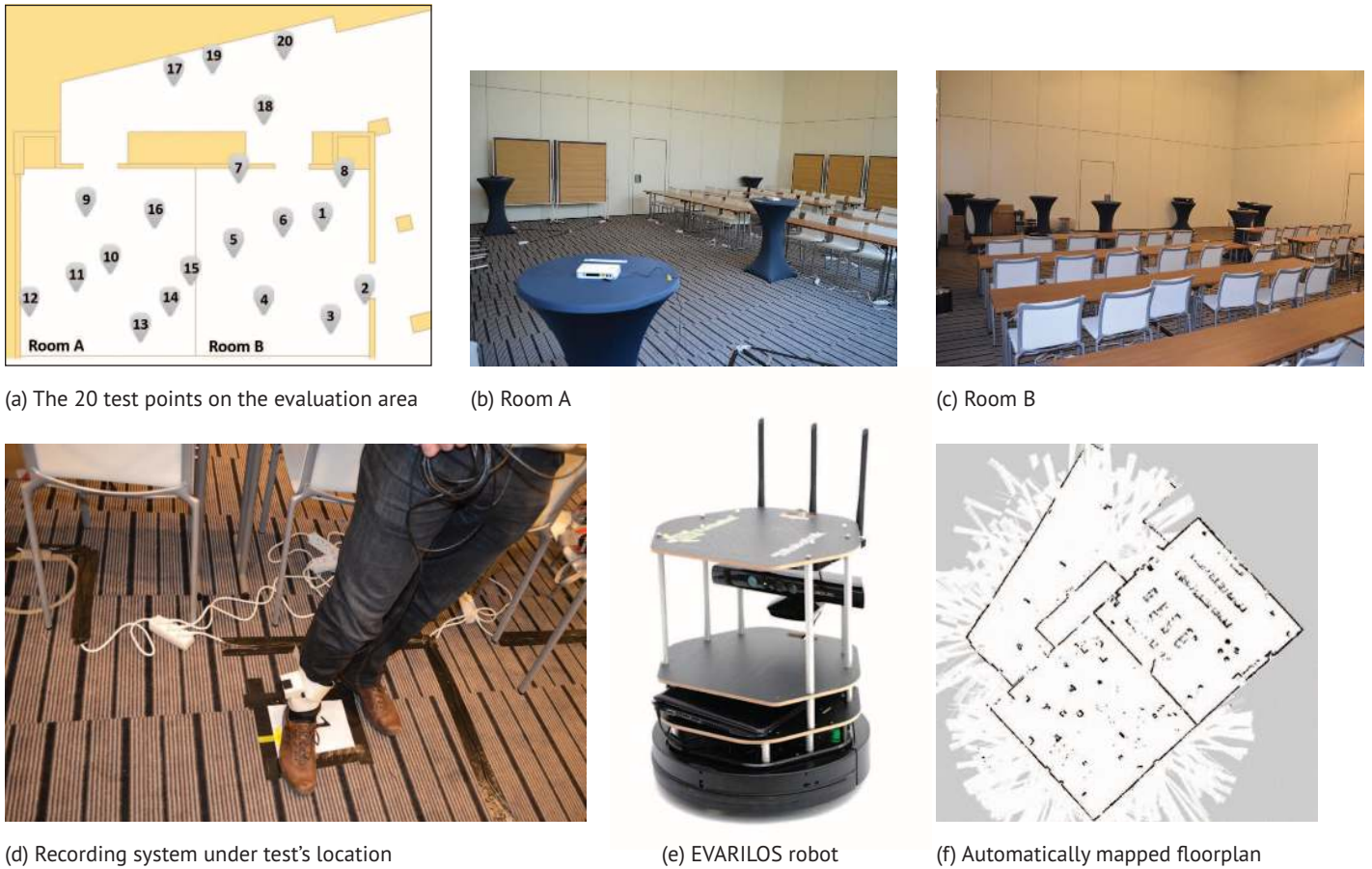
FIGURE 1. The 300m 2 area used for the competition. 20 evaluation points were placed into two rooms and the hallway. Besides the manual evaluation, the EVARILOS robot automatically mapped the competition area and then was used to automatically evaluate the accuracy of the top two teams.
