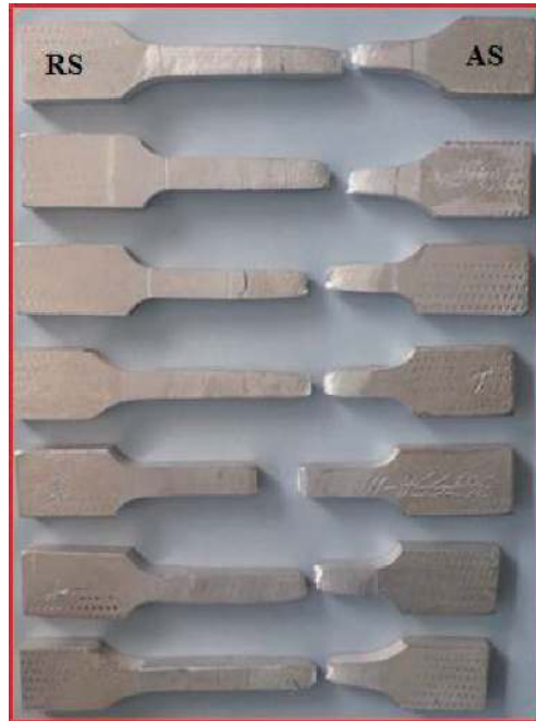
FIGURE 9: Fractography of tensile test specimen.
