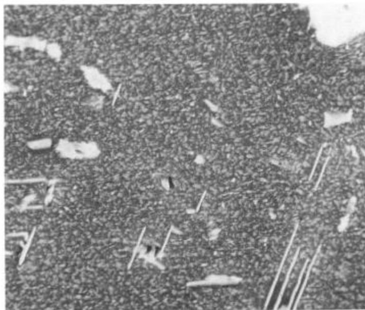
Figure 7 - SEM photomicrograph of alloy 625LCF after exposure at 650°C for 5000 hrs (7 months). There is some coarsening of carbides and a larger quantity of \delta platelets forming. Magnification: 10,000X
