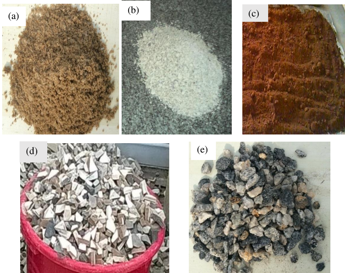
Figure 1. Aggregates used (a) river sand (b) fine ceramics (c) laterite (d) coarse ceramics (e) granite
