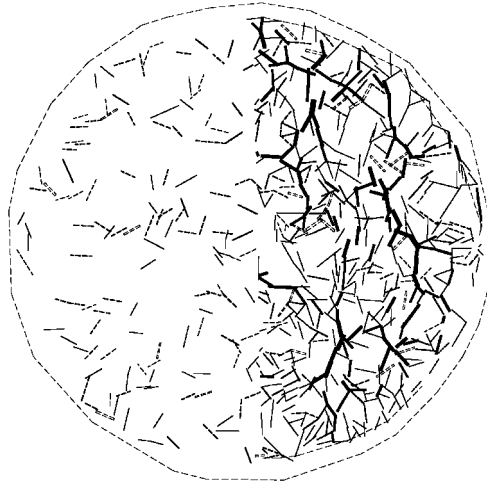
Figure 31. Total forces at the contacts in stress state LC ( \phi_{\text{mov}} = 30^\circ , s = 90 kPa, see Figure 28(a)). The left part of the Fig. shows forces at contacts in which a negative force exists.
