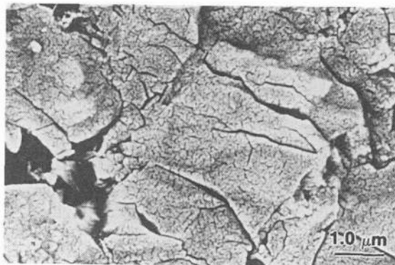
Figure 4. Particle fracture produced by shock consolidation of silicon carbide (initial particle size equal to 7 \mu\text{m} ).
