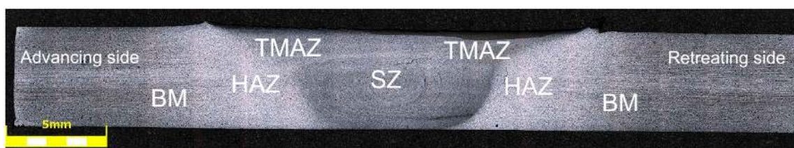
Figure 3. The cross-weld macrostructure of the 5083 FSW weld.
