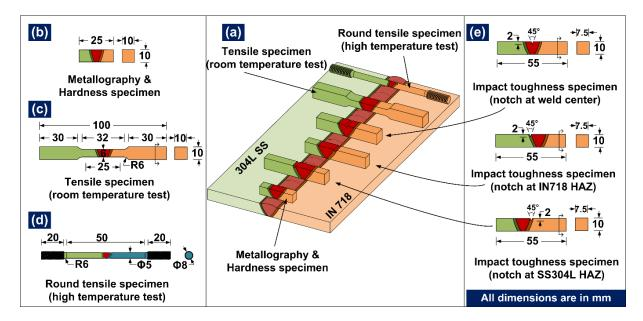
Figure 3. (a) Schematic showing the extraction of test coupons from a welded plate, (b) test coupon for metallographic study, (c) test coupon of room-temperature tensile test, (d) test coupon for high-temperature tensile test, (e) test coupons for Charpy impact testing of weld metal and HAZ.
