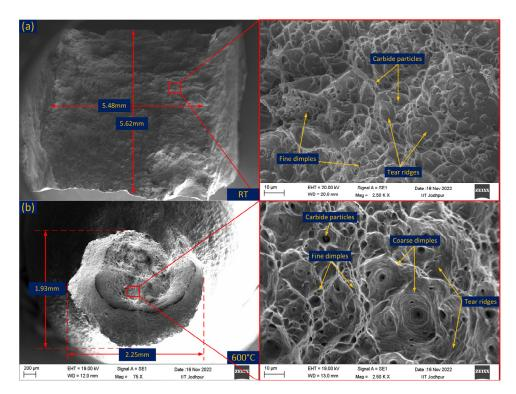
**Figure 11.** SEM image of the fractured tensile specimen tested at (**a**) room temperature (RT), (**b**) at 600 °C (HT).
