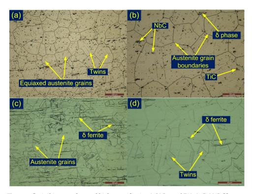
**Figure 1.** Optical image at low and high magnification (a,b) Inconel 718, (c,d) 304L SS.
