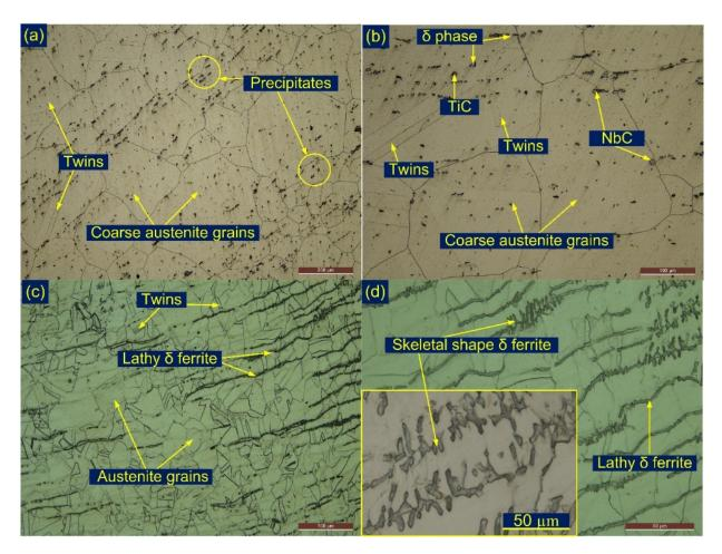
Figure 6. HAZ of IN718 (a,b); 304L SS (c,d).
