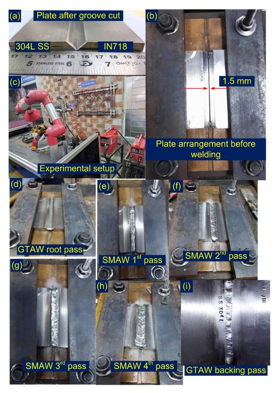
**Figure 2.** (a) Plate after groove preparation, (b) arrangement of the plate before welding, (c) welding machine setup, (d) plate after GTAW root pass, (e-h) SMAW filling passes, (i) backing GTAW pass.
