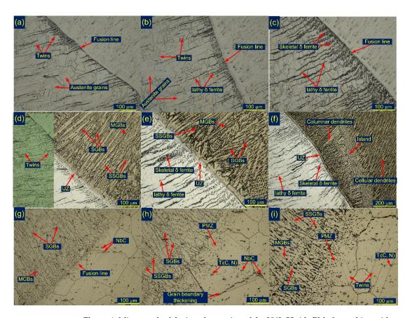
**Figure 4.** Micrograph of the interface region of the 304L SS side BM after etching with aqua regia  $(\mathbf{a}-\mathbf{c})$ ; after electrolytic etching  $(\mathbf{d}-\mathbf{f})$ ; interface on the side of IN718 BM  $(\mathbf{g}-\mathbf{i})$ .
