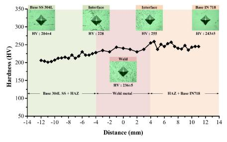
Figure 12. Hardness distribution across dissimilar weldment.
