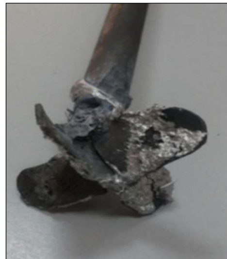
FIGURE 3: The four blades stirrer.
