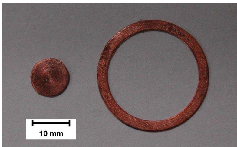
Fig. 2. Appearance of disc (left) and ring (right) samples after HPT for one revolution.
