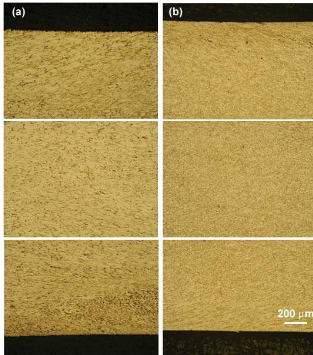
Fig. 7: Longitudinal photomicrographs of as-spray-rolled 2124. (a) Spray rolled at G/M = 0.15 near each rolling surface (top, bottom) and near the center of a 4.3 mm thick strip. (b) Same as (a) but spray rolled at G/M = 0.30 .
