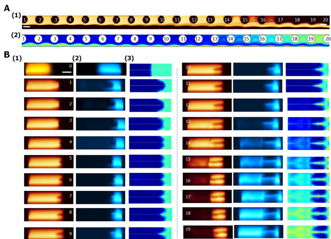
Figure S3. Experimental confirmation of the secondary flow motion with a pillar spacing of 440 \mu\text{m} . A. (1) Fluorescent images from the top view as fluid flows downstream. (2) Corresponding numerical results. Vortices are formed after pillars and particles can become trapped there in some cases. Regardless of particle trapping in the vortices, pillar spacing below 1.1 mm showed lower focusing efficiency. Scale bar represents 200 \mu\text{m} . B. (1) Confocal fluorescent images show the folding of fluorescent dye solution injected with DI water as co-flow (operated at Re = 100 ). (2) Confocal fluorescent images (false color) when dye is introduced in the other half of the channel. (3) FEM simulation results. Scale bar represents 100 \mu\text{m} .
