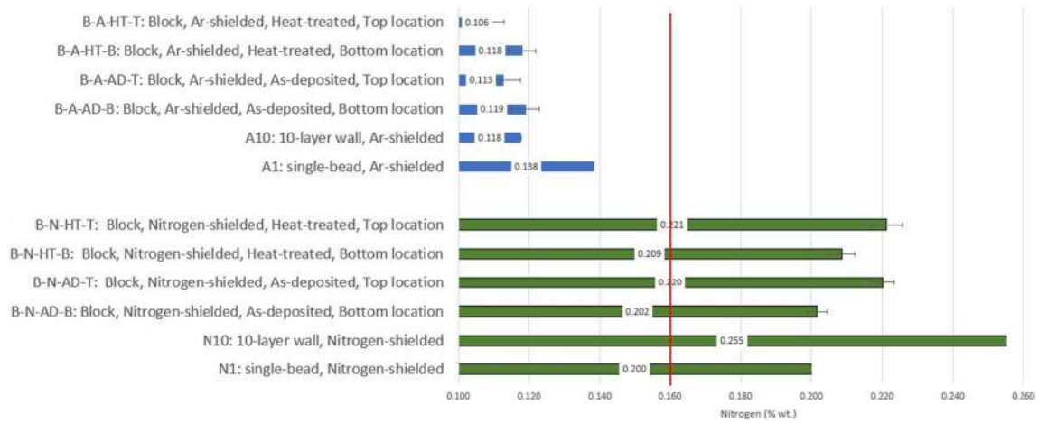
Fig. 6 Nitrogen content (wt%) measured in the single-bead samples (A1, N1), in the 10-layer wall samples (A10, N10) and in the block samples (B-A-HT, B-A-AD, B-N-HT, B-N-AD). The block designations end in T or in B, referring to the location of the measurement and being top and
