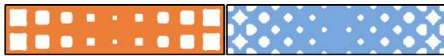
Figure 17: Two gradients computed for the same goal parameters, using geometry (left) and boundary forces (right) to estimate the boundary dissimilarity during synthesis. The actual material parameters for the right structure deviate less from the predicted parameters (error of 0.0266, left, and 0.0137, right).
