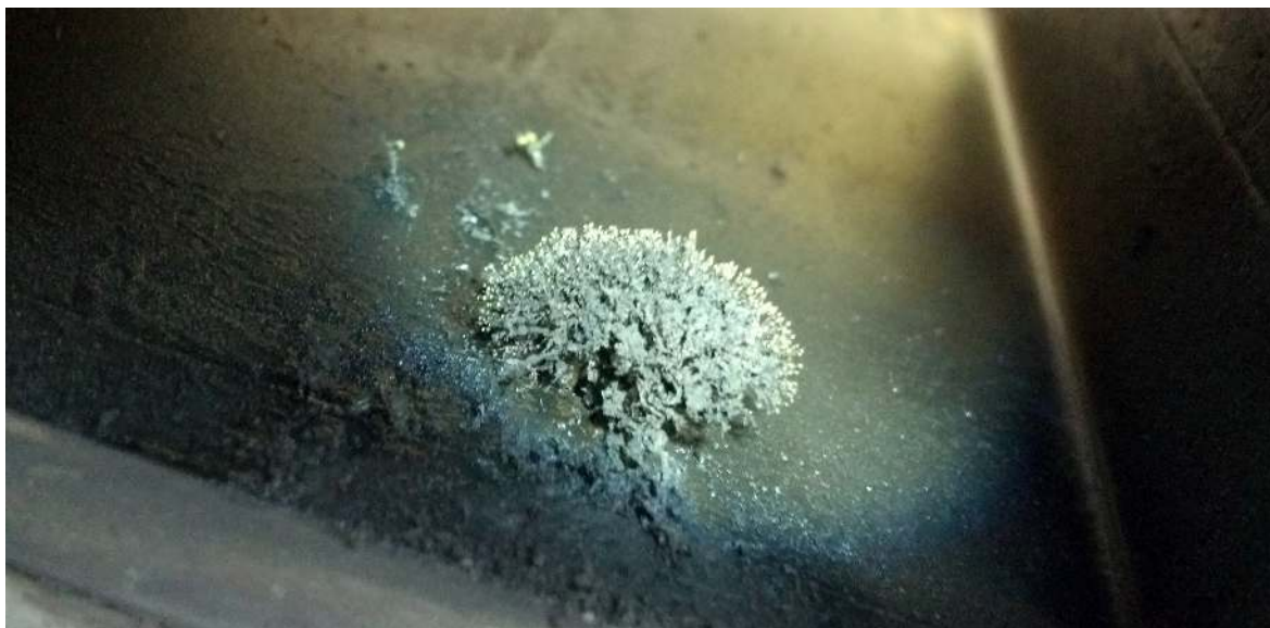
Figure 6.16: Carbon filament formation resulting from the creation of microplasmas in the hydrocarbon pyrolysis gas. The formation shown in this image is approximately 2 cm across.
