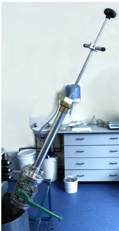
Figure 3.7: Batch addition plunger injection apparatus ready for injection. The PTFE cap at the top end is screwed down creating a gas-tight seal once the sample has been added; an O-ring and ball valve seal the bottom of the system until the sample is injected into the reactor.
