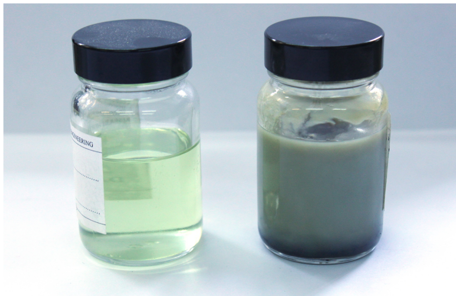
Figure 4.1: Condensed pyrolysis products generated using activated carbon (left) and coke (right) reactor beds. The activated carbon derived condensate is entirely liquid at room temperature and clear — notice that it is sufficiently transparent that the sample label is clearly visible at the rear of the glass sample bottle. The condensate produced using a coke bed, by contrast, is mostly solid at room temperature and entirely opaque.
