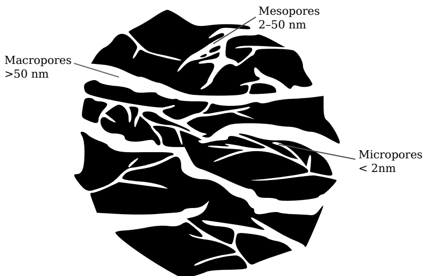
Figure 2.2: Schematic representation of pores in an activated carbon particle. Pores are able to extend deep into a substance in three dimensions, significantly increasing its overall surface area.
