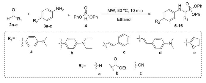
Scheme 1. Synthesis of  $\alpha$ -aminophosphonates 5–16 by MW-assisted KF reaction.
