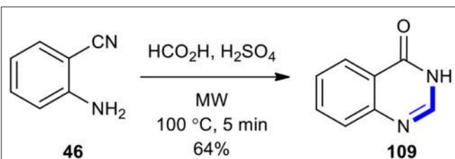
SCHEME 50 | MW-assisted synthesis of 109 from 46 and formic acid.
