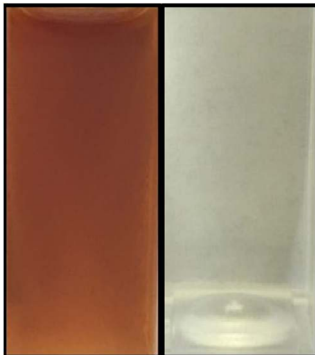
Figure 4. Dark brown-reddish color of the reaction mixture (Left) after a reaction time of 4 h using cellulose and a borosilicate glass reactor containing 1645 ppm HMF and 125 ppm levulinic acid (Right) Transparent color of a standard solution of 2000 ppm HMF and 2000 ppm levulinic acid.
