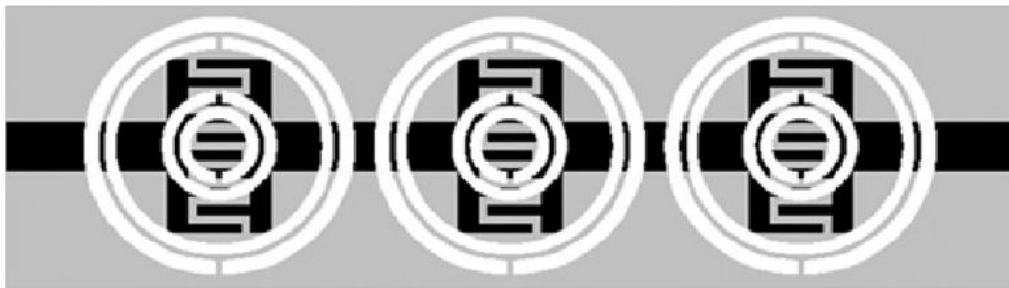
Figure 7.5. Ultra-wide band-pass filter geometry [127]
