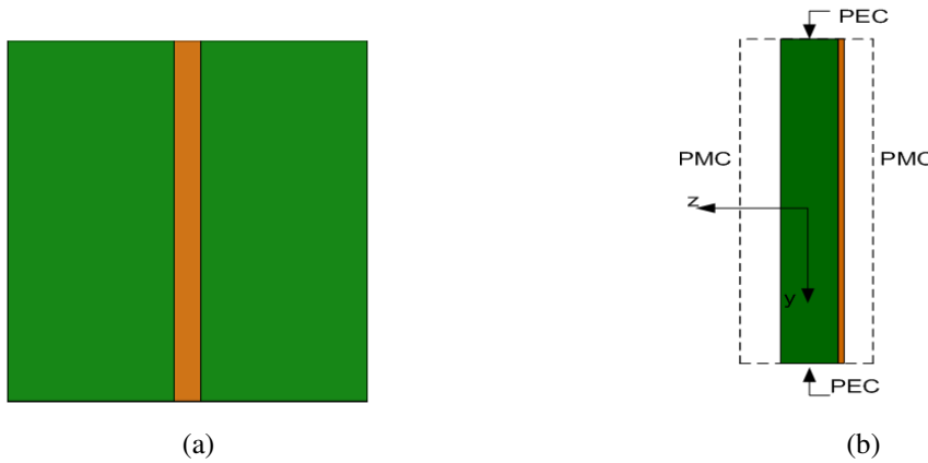
Figure 4.8. (a) One unit cell of wire strip geometry (b) boundary conditions imposed on the edges of one unit cell
