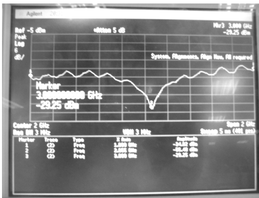
Fig. 16. Measured Power Transmission (1 - 3GHz).
