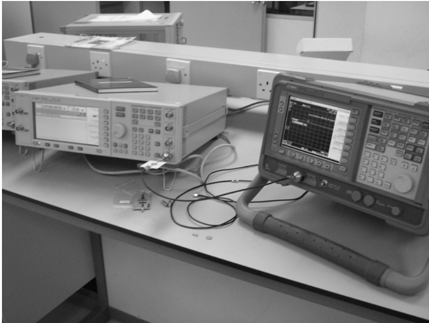
Fig. 12. DRF Power Transmission Measurement Setup.
