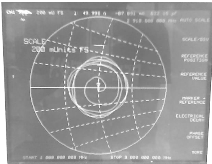
Fig. 8. Measured Input Impedance of DRA Structure.
