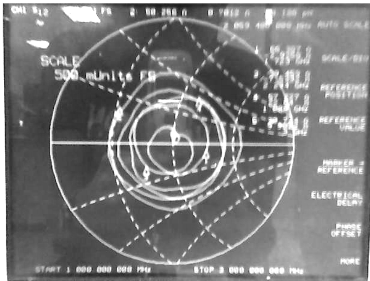
Fig. 18. Measured Impedance Response of Structure.
