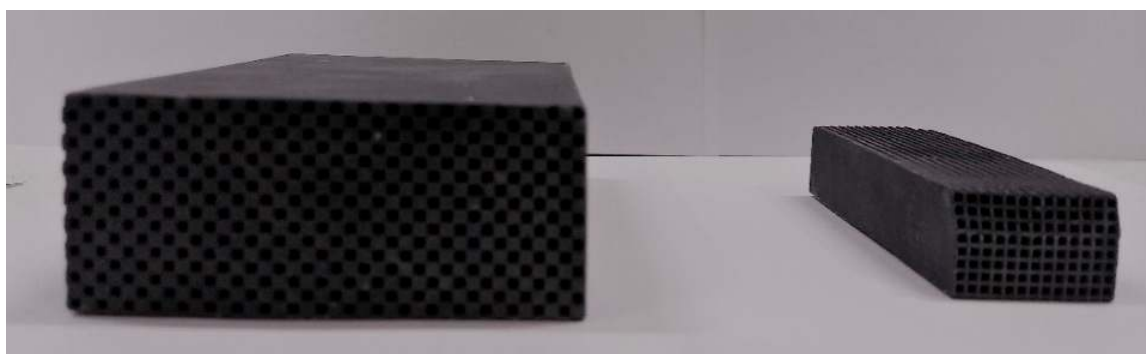
Figure 8. Silicon carbide monoliths, wall-flow type (left) and flow-through type (right).
