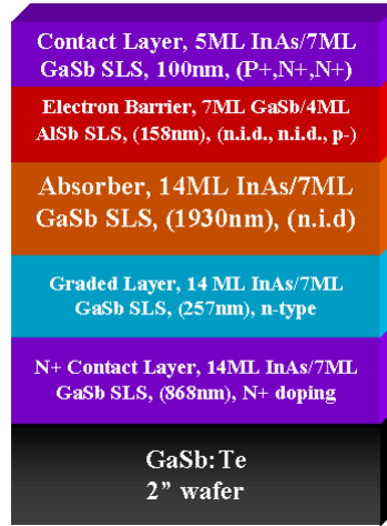
Figure 6.1: Schematic of the LW pBn, nBn, and nB(p-)n structures.
