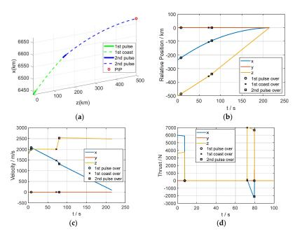
**Figure 3.** Curves of the state and control variables of the interceptor in scenario 1: (**a**) trajectory, (**b**) relative position, (**c**) velocity, and (**d**) thrust.
