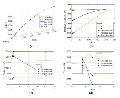
**Figure 4.** Curves of the state and control variables of the interceptor in scenario 2: (**a**) trajectory, (**b**) relative position, (**c**) velocity, and (**d**) thrust.
