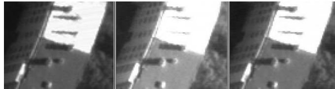
Figure 14: First extract of the stereo pair. From left to right : in the original image, in the specified one, in the equalized image.
