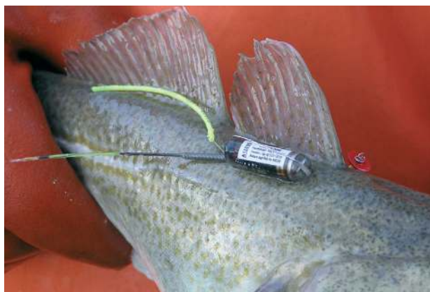
Fig. 2. Gadus morhua . External attachment of an archival tag to a fish. Anterior and posterior wires of the tag have been tied up separately
