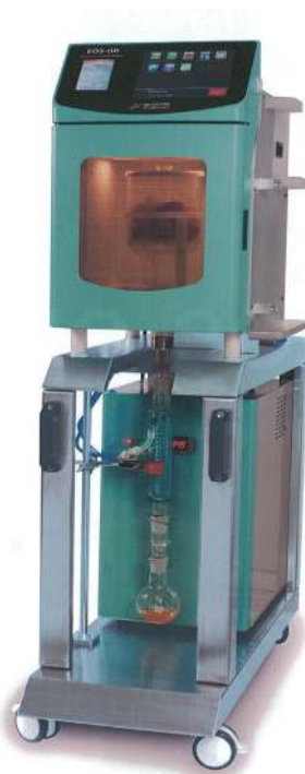
Slika 3. Uređaj za mikrovalne ekstrakcije i hidrodestilaciju s gravitacijom (Bousbia i sur., 2009) (Zahvaljujući prof. Farid Chematu i Milestone Technologies (EOS-GR, Milestone Tecnologies)) Fig. 3. Apparatus for microwave extraction and hydrodistillation with gravity (Bousbia i sur., 2009) (Thanks to prof. Farid Chemat and Milestone Technologies (EOS-GR, Milestone Tecnologies))
