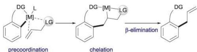
Scheme 68 Proposed general mechanistic steps of the coordination-assisted allylation.
