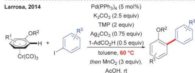
Scheme 46 Substrate activation by Cr 0 complexation in catalytic direct arylation. 110,111 TMP = 2,2,6,6-tetramethylpiperidine.
