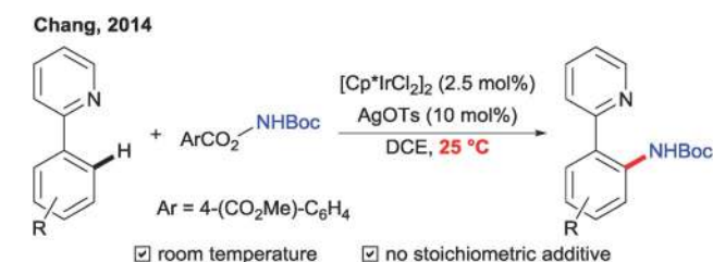
Scheme 56 Mild Ir-catalyzed amination with an electrophilic reagent. 123
