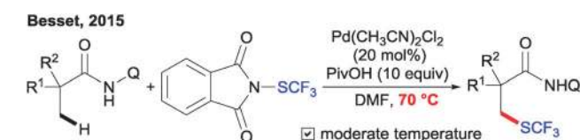
Scheme 33 \text{C}(\text{sp}^3)\text{-H} trifluoromethylthiolation with a bidentate DG. 83
