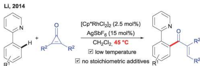
Scheme 64 Chalcone synthesis using cyclopropanones. 132
