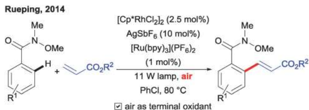
Scheme 76 \text{Rh}^{\text{III}} -catalyzed oxidative olefination using photoredox catalysis to replace stoichiometric amounts of oxidant with air. 156
